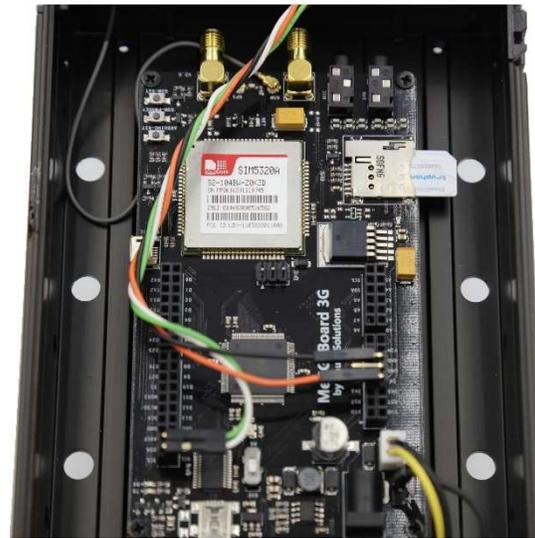
The photo on the left shows the Communicator drive tray with the cover removed, it's important to note the location of the SIM card slot to the left of the SIM5320 Chip.
