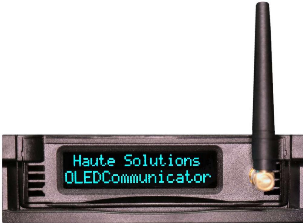
This is a photo of the front of an OLED Communicator as it might be installed in a PC. Note that the antenna is threaded and should be removed from the drive tray prior to insertion or removal from the system. The antenna will perform well with the threaded connection seated finger-tight.
