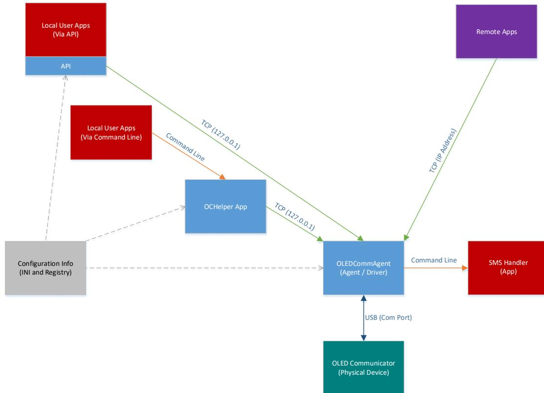
**OLEDCommAgent:** Basic functionality of the OLED Communicator is handled via an Agent (driver). The Agent (*OLEDCommAgent.exe*) communicates with the OLED Communicator hardware via serial protocols over a USB connection. The Agent acts as a message and protocol handler for the Communicator. Generally, all communications to/from the Communicator should be handled by the Agent!
