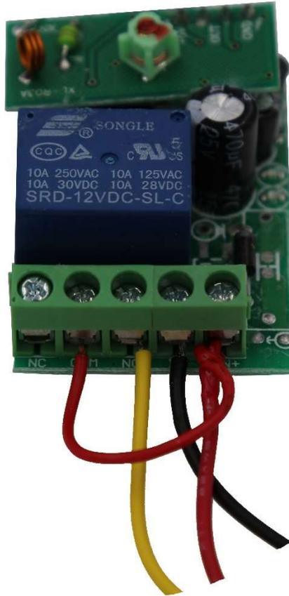
Red Wire: Connect to Battery Positive Power Supply (12V+)
