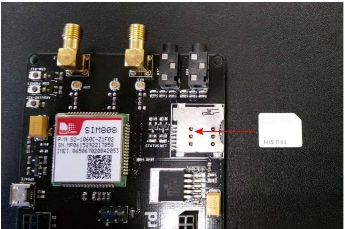
(The upper board has been removed in the photo to aid in clarity. We do not recommend separating the two boards as it is quite easy to misalign the upper board during reinstallation. Note that this is an older PCB in the photo although the SIM Card Orientation is identical.)
