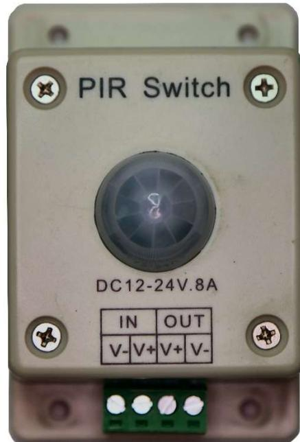
IN V- : Connect to Chassis Ground or Battery Negative (12V-)
