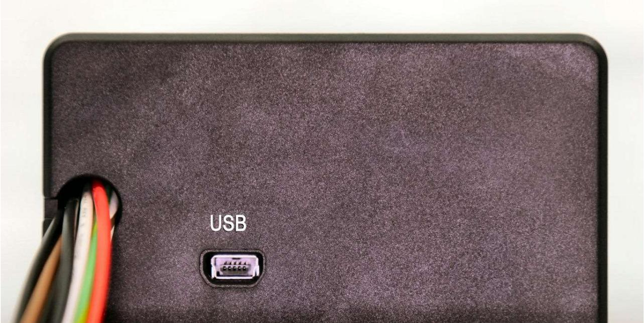
On the other end of the enclosure we have the USB port used for programming and updating the alarm.
