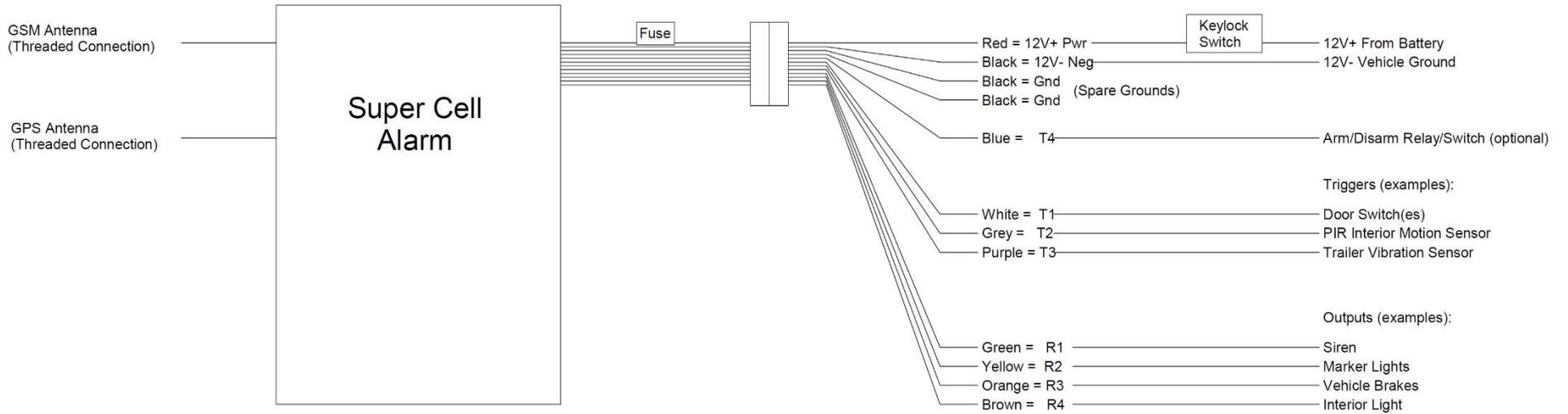
**Accessory Wiring:** Here is a schematic which shows specific terminal/wiring assignments: Note that this diagram reflects the alarm using the default factory configuration and illustrates connections for specific optional accessories.
